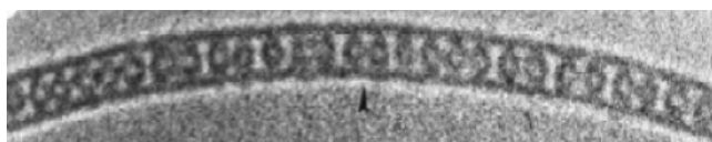
Figure 80. High-resolution TEM image of one of the first C 60 @SWNCTs (peapod) ever observed. The carbon nanotube diameter is that of a regular (10,10) SWNT (14 Å). Reprinted with permission from ref 264. Copyright 1999, Elsevier.
